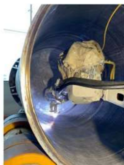
Execution of the weld overlaying on the W1C circular joint
