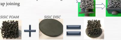
Development of a brazing process suitable for the production of Si-SiC solar receivers
