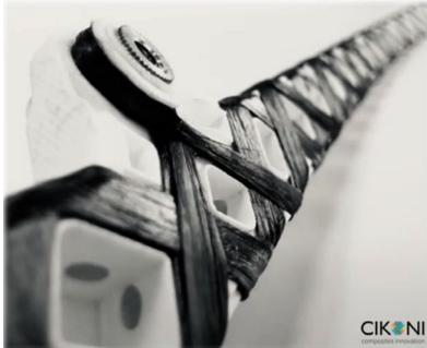
**Additive Manufacturing + Thermoset Winding**
