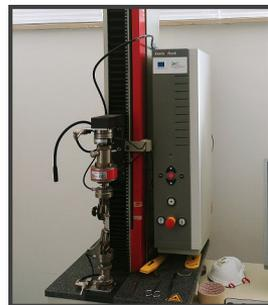
Tensile test machine on single filaments
