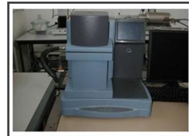
DMA Instrument (Q800 TA Instrument)
