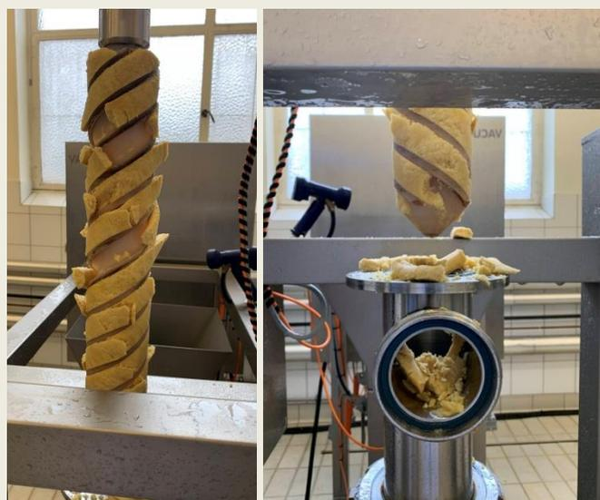
*Our pilot-scale spiral filter press, which can process 40 L of apple cell culture and capture 1–2 kg of cell biomass.*
