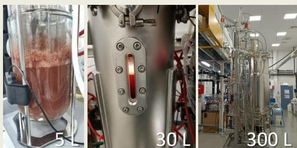
*Dragon fruit cell suspension cultures in large-scale bioreactors, from 5 to 300 litres.*
